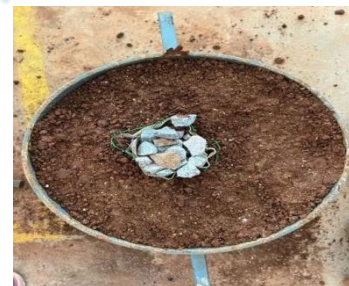
Fig 5: column filled with stone+ m-sand +coconut shell.
